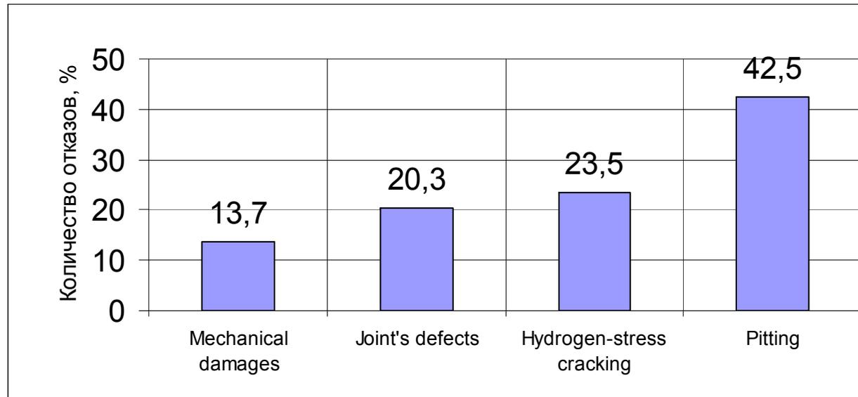
The analysis\* of a plenty cumulated datas for the operational period of OrenburgGasprom from 1974 till 2005, allows to allocate corrosion process as a determining type of pipeline damages. And pitting is the main component of this process.
